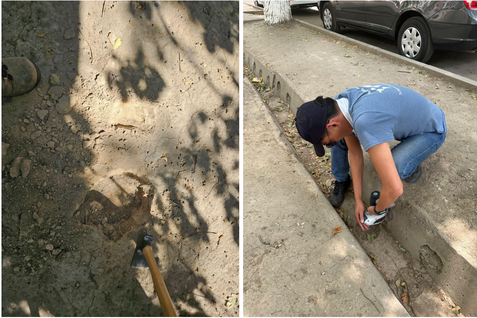
Left: Another example of prepped test pits at surface level, 3 cm, and 10 cm in a playground. Right: This is an example of canals that run through some parks. Older soil gets trapped inside, so the XRF was used to measure the concentration of this older soil.
