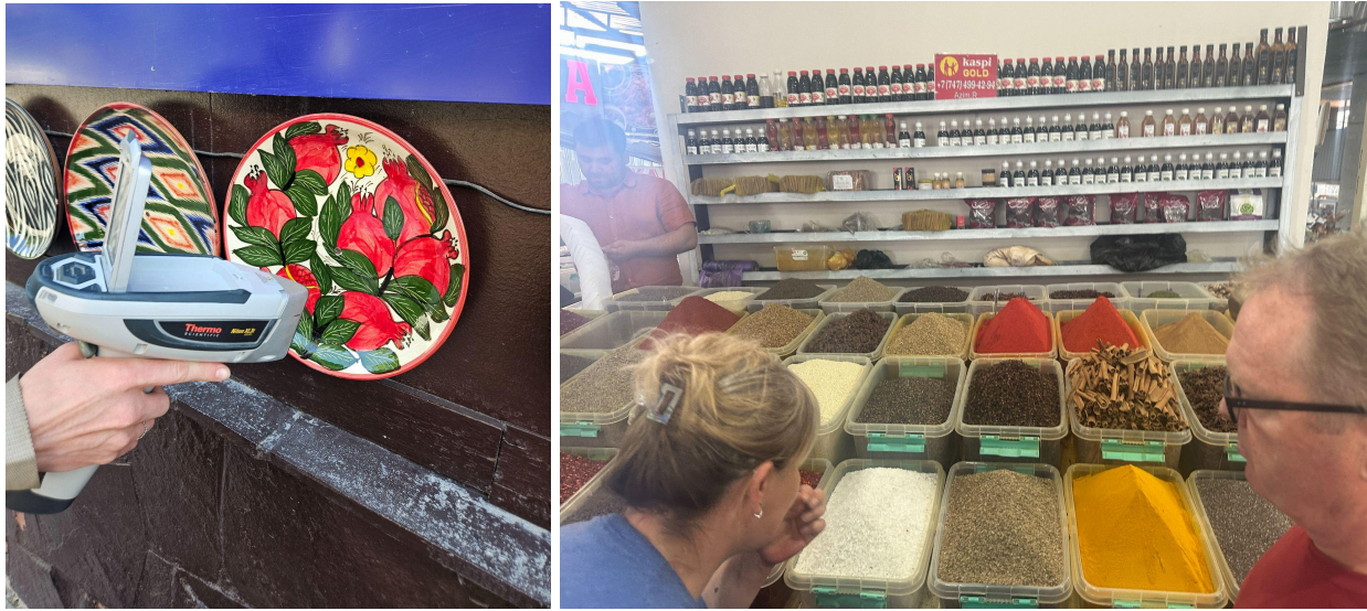
Left: Ornamental plates were tested by the XRF and were found to have high lead levels. This is likely in the glazing used to seal the pottery, but can also come from the use of lead-based paints. Right: A variety of spices were sampled from local vendors.
